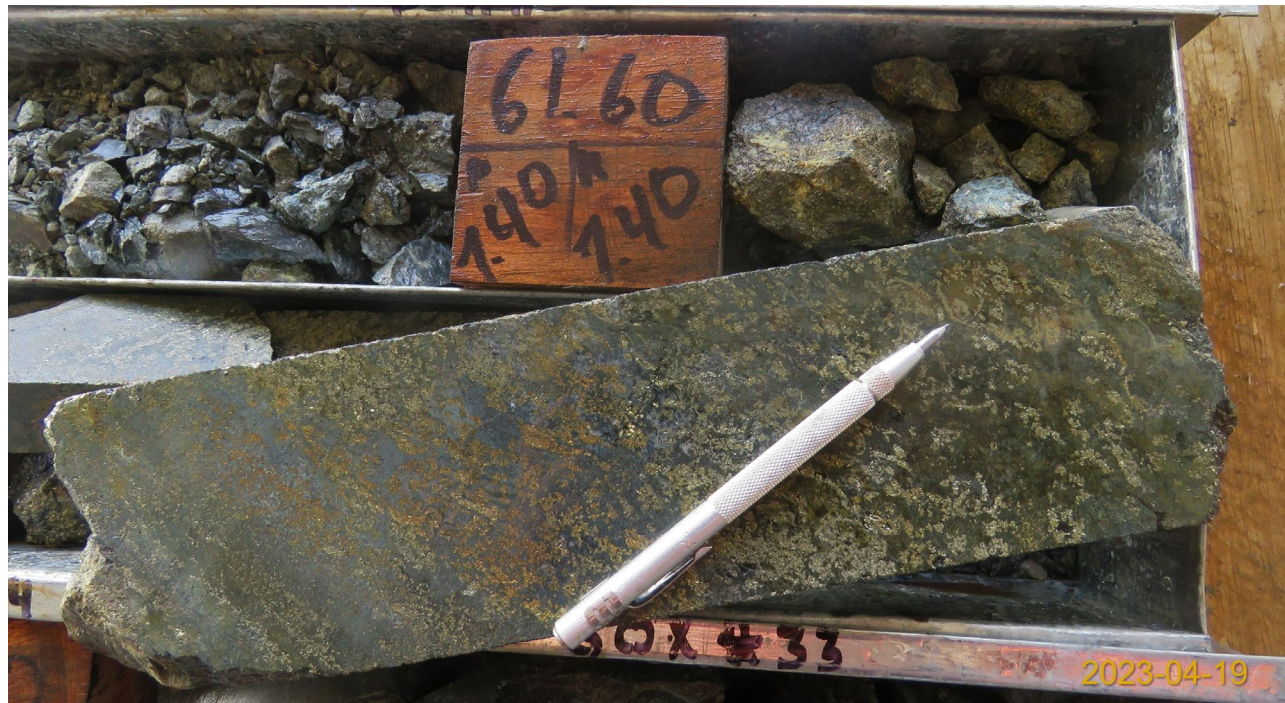
Figure 7: ACD174 at 62.5 m down hole – a fossiliferous limestone bed that is highly replaced by semi-massive sulfides consisting of pyrite, chalcopyrite and trace magnetite. The sample outlines some of the bivalves whose carbonate shells have been preferentially replaced. The host limestone protolith shows pervasive chlorite alteration. This sample was part of 1.8 m interval between 62 m and 63.8 m that returned 1.39% Cu, 0.46 g/t Au and 8.85 g/t Ag.
