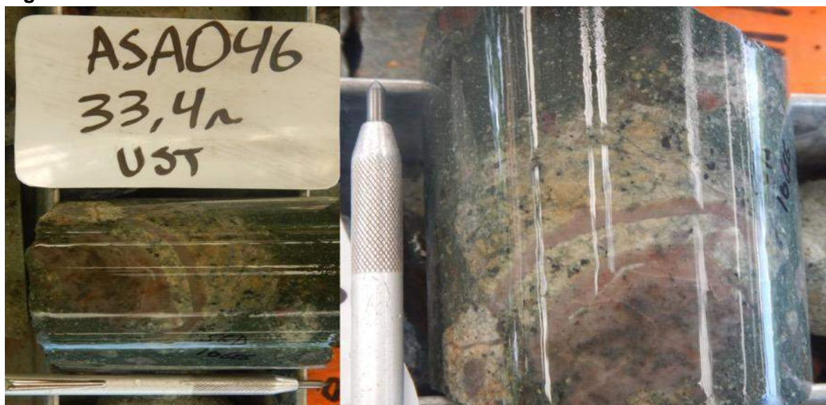
Figure 9: Unidirectional Solidification Textures.
