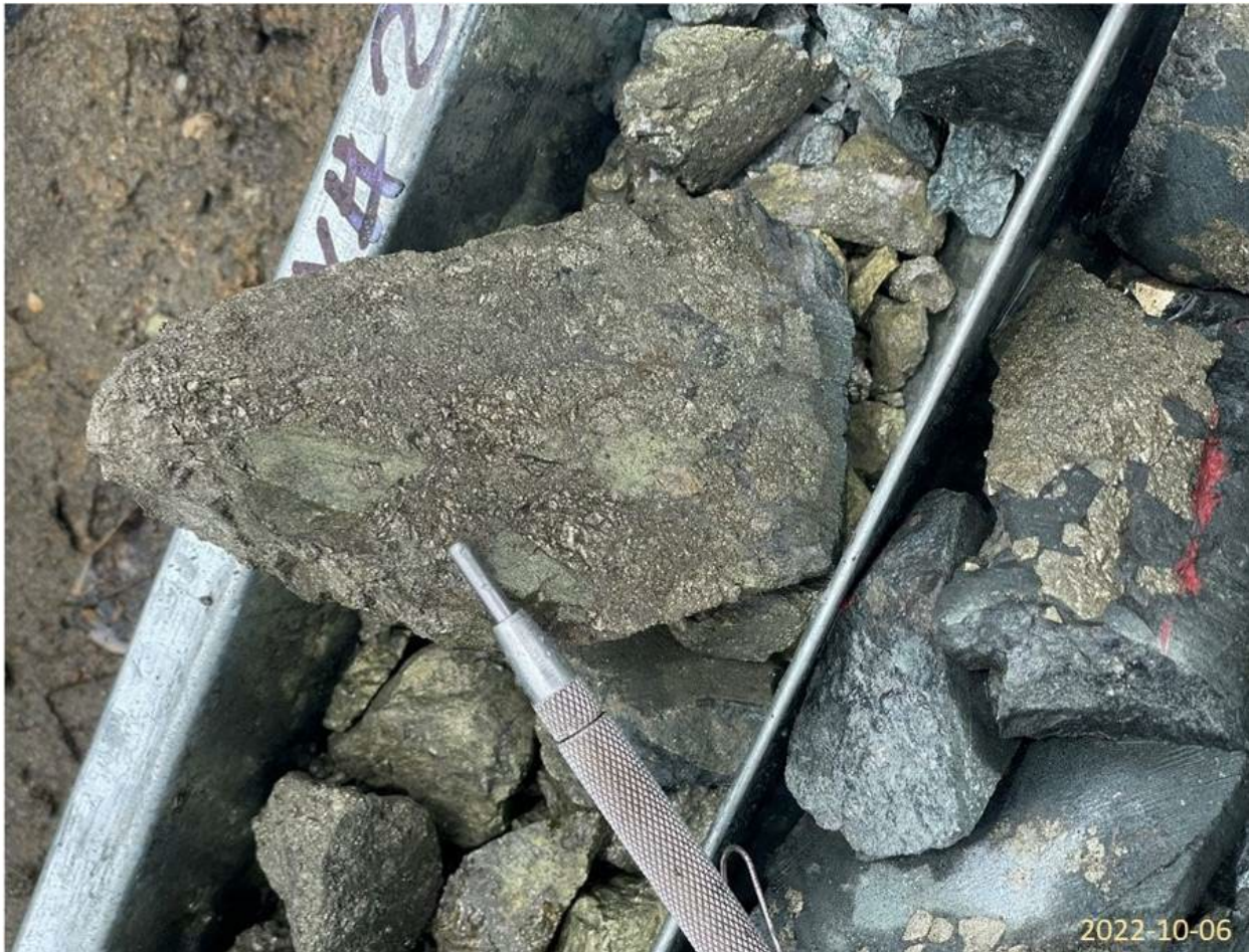
Figure 3: Hole ACD126 also locally intersected massive sulfide replacement of carbonaceous mudstones at 71.30 m, which returned 7.41% Cu, 1.43 g/t Au and 52.4 g/t Ag, or 8.04% CuEq 1 over a 1.40-m interval.
