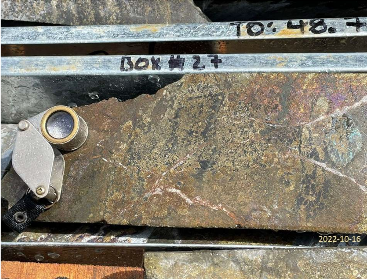
Figure 2: Hole ACD115 at 49.10 m showing local semi-massive sulfide replacement of carbonaceous mudstones that has resulted in high-grade mineralization. This sample was part of a 1-m sample from 48.50 m to 49.50 m, which returned 6.37% Cu, 1.78 g/t Au, 47.4 g/t Ag, or 7.05% CuEq 1 .
