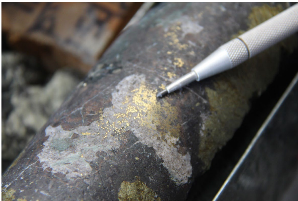
Figure 6: Drill hole ACD036, which returned 0.90 metres of 4,440 g/t gold, 10.25% copper, 24.70% zinc and 347 g/t silver from approximately 112 metres downhole.
