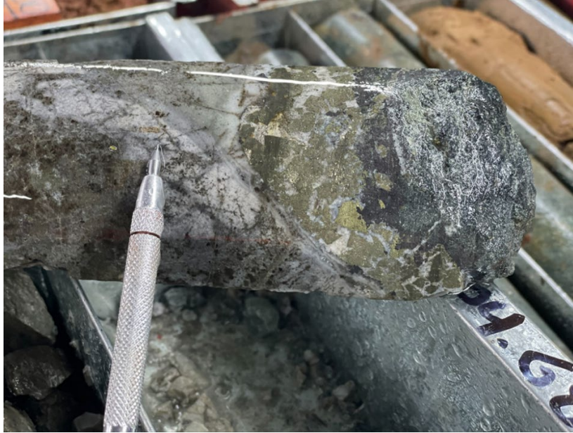
Figure 4: Drill hole ACD114 intersected 0.2 metre of CBM mineralization from approximately 152 metres downhole.
