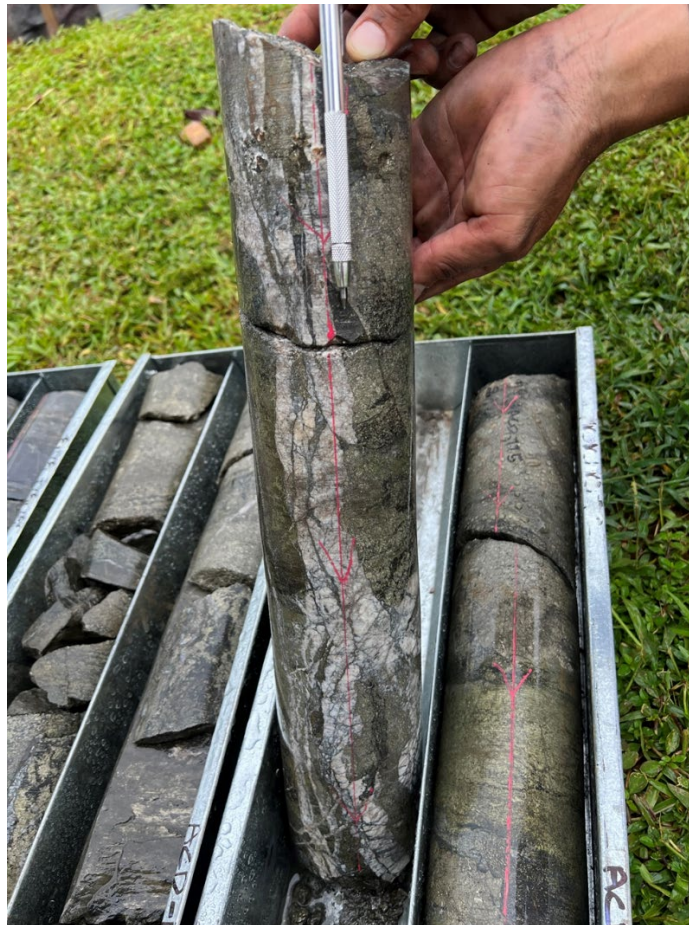
Figure 5: Drill hole ACD115 intersected 0.6 metre of CBM mineralization from approximately 44 metres downhole.
