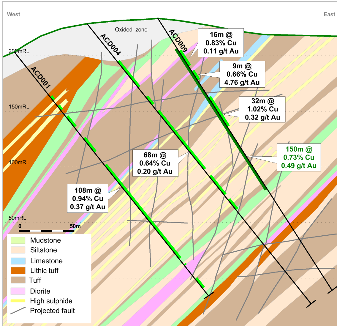
Figure 4. Section 855760mN displaying consistent large widths of copper and gold mineralization between drill-holes on section that extend to surface and remain open down dip.
